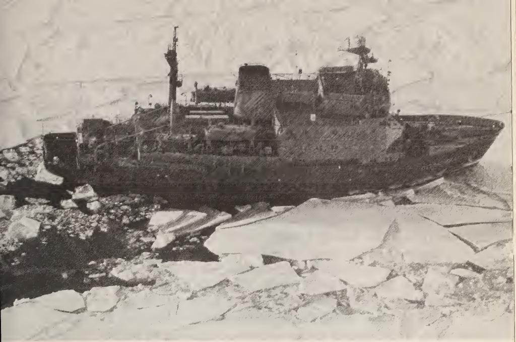
*Icebreaker Otto Schmidt, used to clear the way for cargo ships
